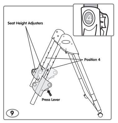
• While pressing the levers on the seat height adjusters, lift them to position 4 on the frame front legs, as shown.
